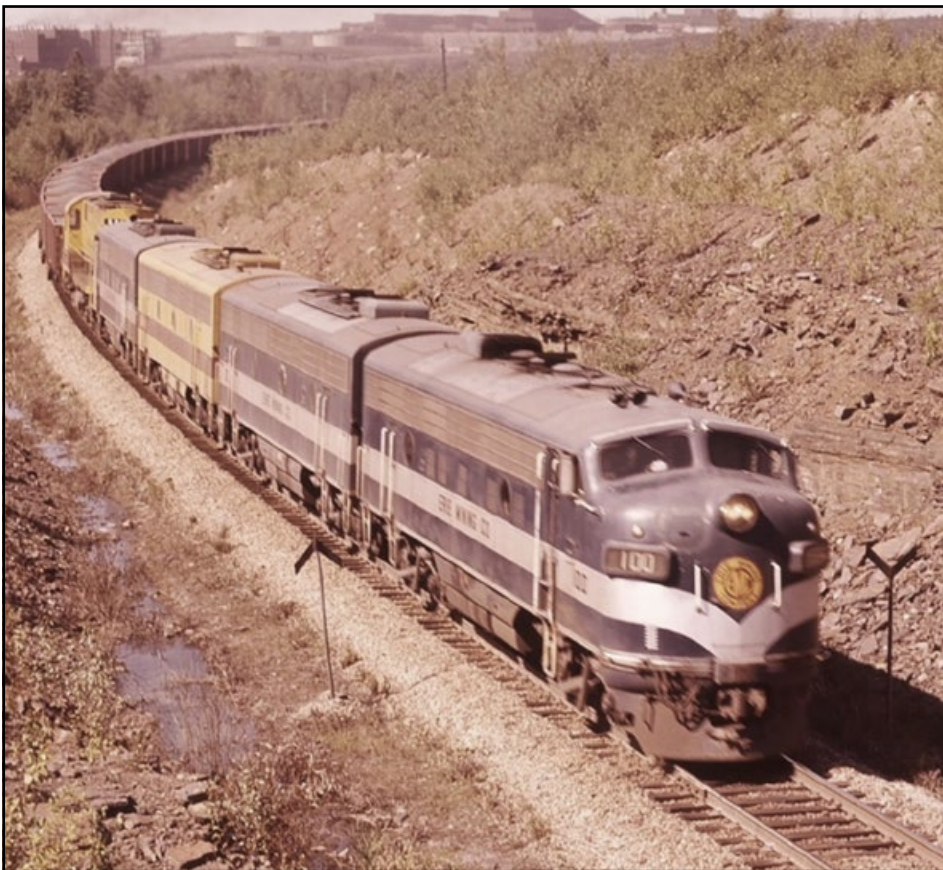
This Model F9, built by the Electro-Motive Division of General Motors, was one of only 87 of its kind. lar ones were frequently used to pull fast passenger trains throughout North America. The F9 was the culmination of locomotive development through the mid-1950s. Based on the highly popular design of stream- lined passenger locomotives, the engine was used in freight service for many years in the Iron Range until acquired by Powell Felix for use on his Vermilion Valley Railroad near Covington, Ind. The historic F9 loco-
