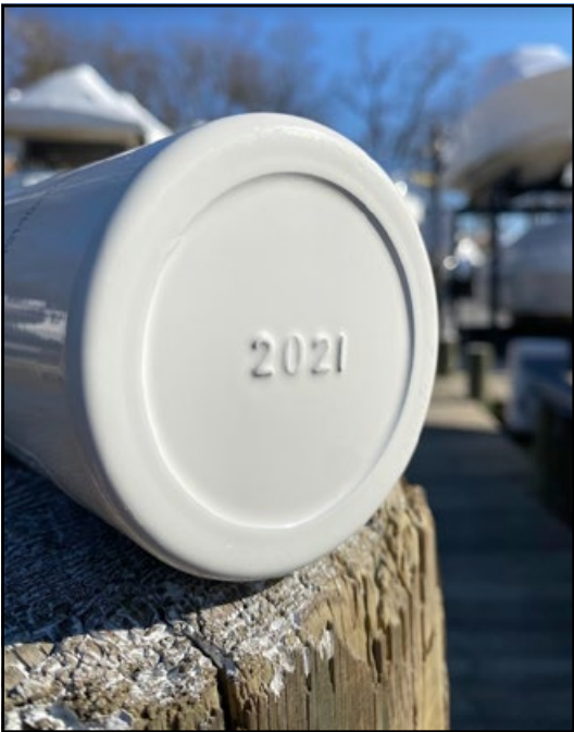
Photos provided by National Safe Boating Council (Left) Boat fire extinguishers expiration date can be two or four digits; if it is two, as in "08," that means 2008. (Right) Engine cutoff switches (ECOS) are often activated by a lanyard connected to the operator that, when pulled, stops the boat's engine.
